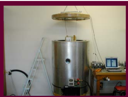
Figure 5: The environmental chamber which is used to test the glider and calibrate the atmospheric measurement sensors.
