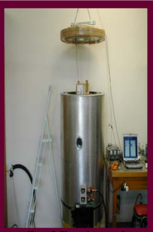
Figure 5: The environmental chamber which is used to test the glider and calibrate the atmospheric measurement sensors.
