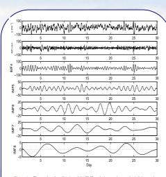
Figure 1 – The results of application of the EMD technique to the zonal wind time series observed by the Scott Base radar at 90 km in January 2006 are displayed. The upper panel in this figure displays the original time series. The second panel contains the summation of the first to third IMFs, the third panel contains the fourth IMF, the fourth panel the fifth IMF etc.
